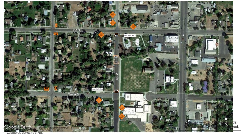
B) SHOULDER, ONE-LANE, TWO-WAY AND DOWNSTREAM TAPERS: USE A MINIMUM OF 1 DEVICE PER 3 FEET OF WIDTH (OR PORTION THEROF). pLUS 1 ADDITIONAL DEVICE TO START.
